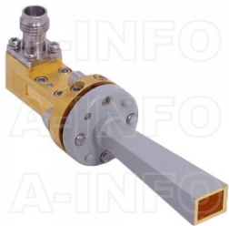
LB-15-10-C-1.85F Standard Gain Horn Antenna 50-65GHz 10dB Gain 1.85mm Female
